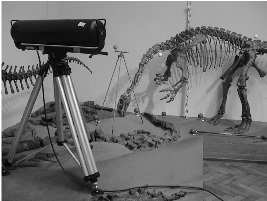
Figure 3: Scanner setup with dinosaur skeleton and reference points
