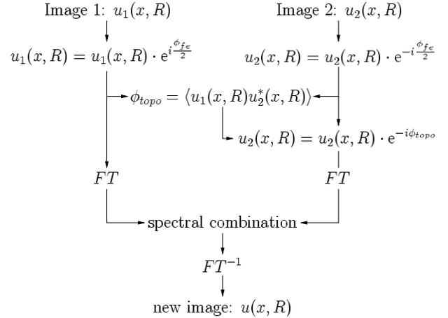
Fig. 2. Block diagram of the proposed superresolution algorithm.
