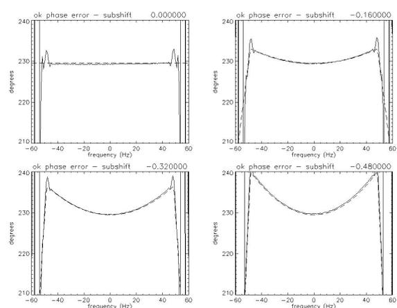
Figure 6: Phase response of a simulated point target in frequency domain using parameters of Table 1, with different subpixel shifts (16%, 32% and 48% of the range sampling interval) when the mapping range is smaller than the real range of the target. The dashed line illustrates the theoretical phase error expressed by equation 3. From this figure becomes clear that the measured digital error coincides with the error calculated by equation 3.
