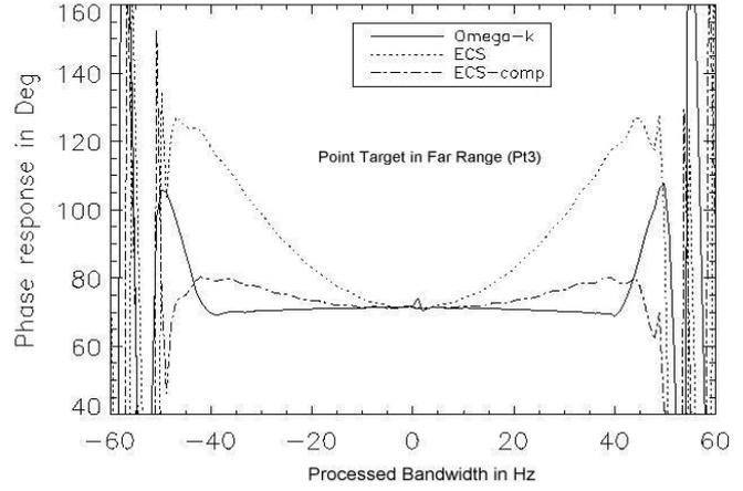
Figure 2: Phase response of simulated far range point target in frequency domain. The residual phase error reduces from  $55^{\circ}$  to less than  $10^{\circ}$  after the correction implemented at the standard ECS processing algorithm.
