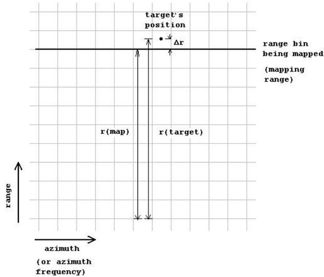
Figure 4: The processed grid of the data (cross sections of the horizontal with the vertical lines correspond to the pixels of the image). The range distance between the target (position of the target's response maximum value, in a subpixel level) and the range where the mapping takes place can be distinguished.
