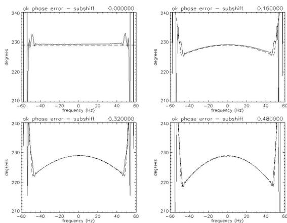
Figure 5: Phase response of a simulated point target in frequency domain using parameters of Table 1, with different subpixel shifts (16%, 32% and 48% of the range sampling interval) when the mapping range is greater than the real range of the target. The dashed line illustrates the theoretical phase error expressed by equation 3. From this figure becomes clear that the measured digital error coincides with the error calculated by equation 3.
