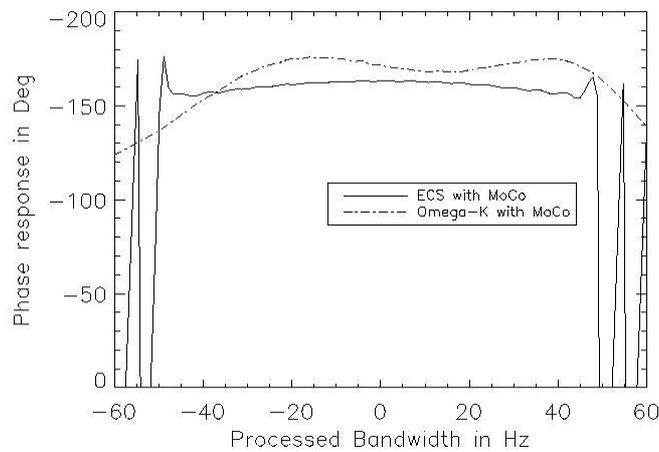
Figure 8: Phase response of one simulated point target located in the center of the processed scene, with motion errors in frequency domain. The Omega-K algorithm fails to compensate even small motion errors resulting to a maximum residual phase error of  $45^\circ$ .
