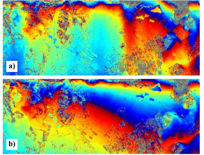
Figure 2. Flattened phase before (a) and after (b) applying the proposed correction method.
