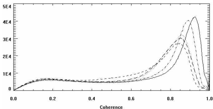
Figure 3. Coherence histograms with different subaperture configurations. Original Coherence (dashed), center  $\pm 7.5$  Hz and bandwidth 30 Hz (solid), center  $\pm 30$  Hz and bandwidth 60 Hz (dash-dot), center  $\pm 50$  Hz and bandwidth 100 Hz (dotted), interpolated using [3] (long dashes).
