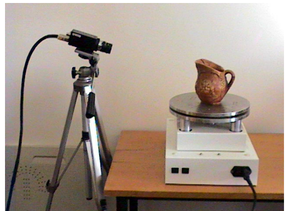
Figure 1: Image acquisition system consists of a turn table, a camera and a computer.
