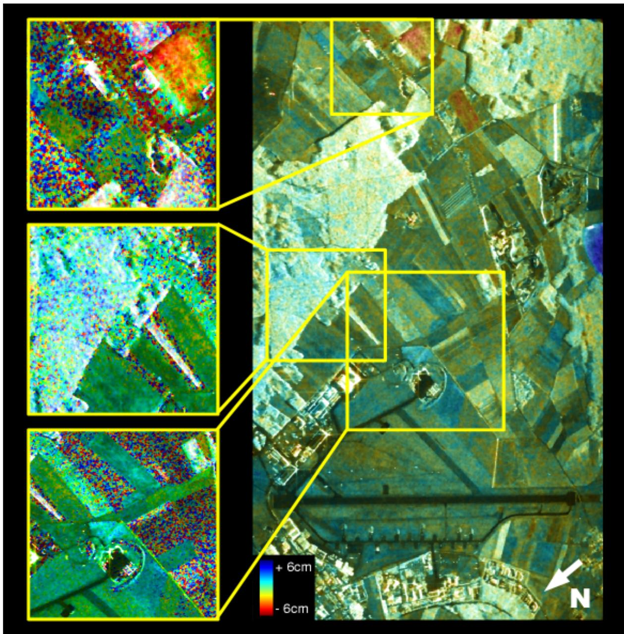
Fig. 1. Overlay of SAR amplitude (magnitude) and differential interferogram (colour) obtain at the Oberpfaffenhofen test-site, obtained by using the coregistration integration method. Temporal baseline: 336 days. The differential phase corresponds to displacements in line-of-sight direction from -6cm (red) to +6cm (blue). Left side: Magnification of 3 areas of interest.
