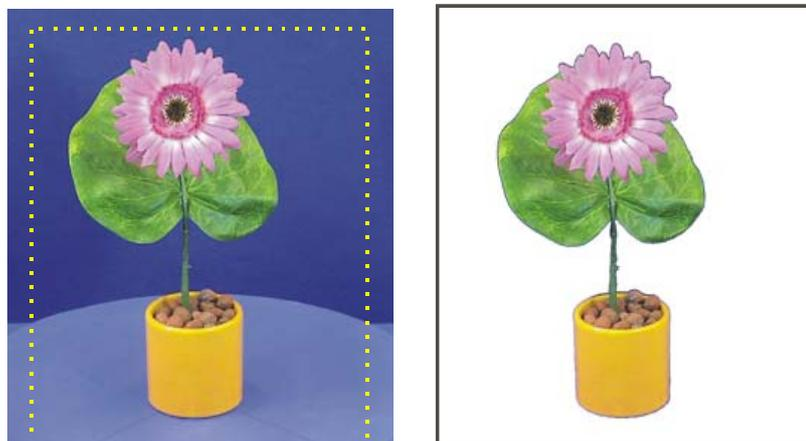
Figure 4: Background estimation using an IHS color space histogram (left) and the resulting silhouette extraction (right).
