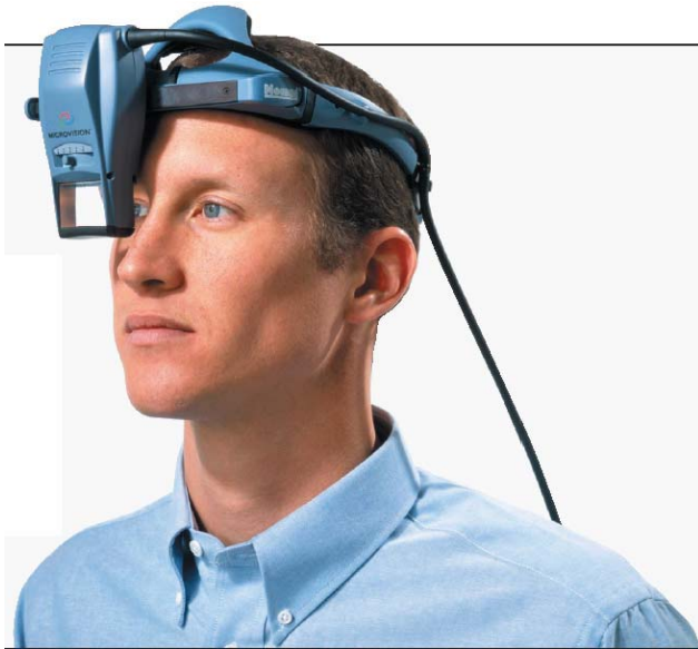
Figure 7. Virtual Retinal Display: Nomad Personal Display System made by MICROVISION
