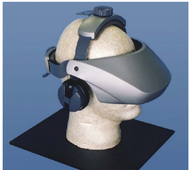
Figure 4. Conceptual diagram of a video see-through HMD (Azuma, 2001)
